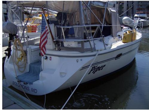
LOA 34'3", LOH 32'6", LWL 28'0", BEAM 11'9", DRAFT 4'4" wing keel. Yanmar 3 cylinder diesel, 29 HP with 1000 hours that is over powered and really pushes her. Fuel capacity 19 gallons, fresh water capacity 51 gallons, hot water heater 5 gallons, holding tank 20 gallons. Charles 30 amp battery charger (2014) and portable 850 watt inverter. Maxwell anchor windlass, 35# CQR with 75' chain, 150' rode and 22# Bruce claw anchor.
